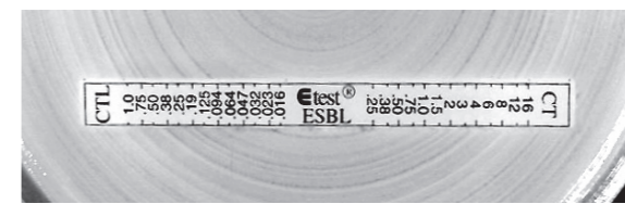
Figure 7. When MIC values are above the test ranges, the result is Non-Determinable (ND).
